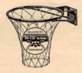
No. 17W—Steel brackets and braces, with official size, 18-inch ring of 5%-inch round steel; steel wire die-formed "NO-TIE" net holder on underside of ring for attaching net, as shown in inset. Electrically welded to one piece. Baked black enameled. Complete with No. 42 thread nets and 8, 2½x%-inch machine bolts.
