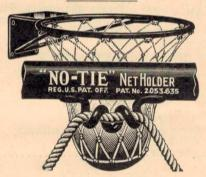
No. 15W—Steel brackets and braces, official size, 18-inch ring of %-inch round cold rolled steel with reinforcement bar on lower side at rear; steel wire die-formed "NO-TIE" Net Holder on underside for attaching net, as shown in inset. Braces streamlined with ring so as not to interfere with close-up shots. Baked black enameled. Heavy No. 60 thread nets and 8,  $2\frac{1}{2}x\frac{3}{8}$ -inch machine bolts. Maximum strength and rigidity—electrically welded to one piece.
